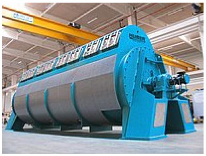
The HUBER RotaDry® Disc Dryer is designed for homogeneous partial drying of dewatered sewage sludge. Due to its compact design and high specific water evaporation, it is not only ideally suited for use in new sewage sludge mono-incineration plants, but also for capacity expansions of existing plants. The dryer can dry exactly to the required DR content and thus enable a self-sustaining combustion in the fluidized bed incinerator.
