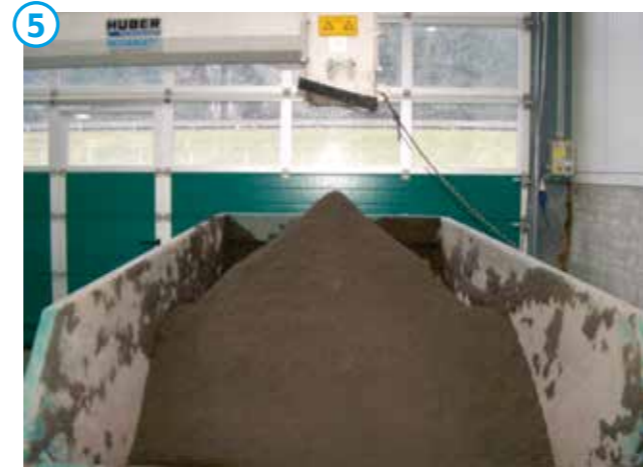
5 Flotate and sediment sludge dewatering with HUBER Screw Press S-PRESS, DR > 50%.
