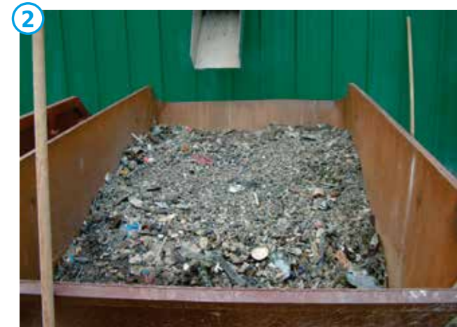
2 Separation of washed out coarse material > 10 mm with HUBER Wash Drum RoSF9.
