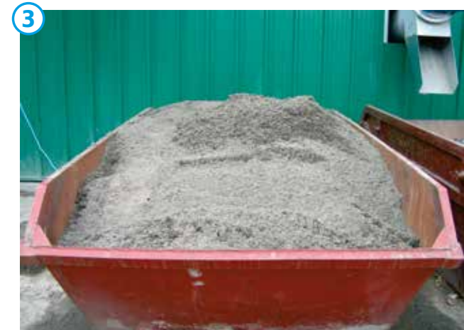
3 Grit from HUBER Coanda Grit Washer RoSF4 DR > 90%, loss on ignition < 3%.
