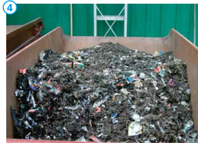
4 Grit from ROTAMAT® Rotary Drum Fine Screen Ro2 DR > 30% (> 1 mm).
