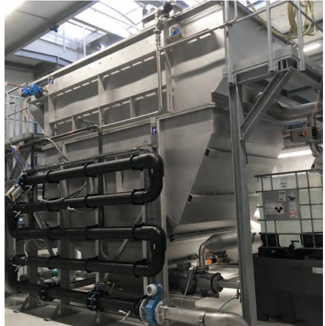
HUBER Dissolved Air Flotation Plants with chemical pre-treatment – full, partial or secondary treatment of industrial wastewater
