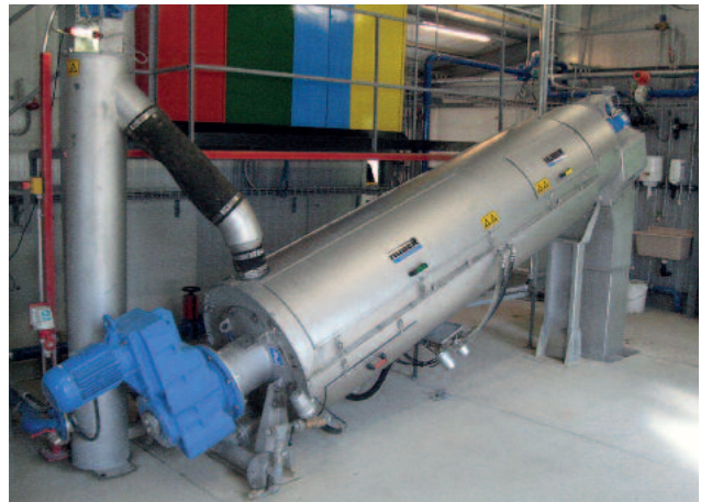
HUBER Screw Press S-PRESS Specific power consumption < 0.01 kWh/kg DR
