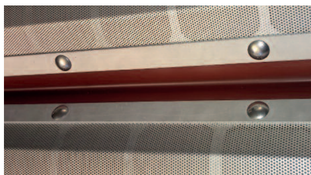
The special sealing system ensures that no unscreened wastewater passes the HUBER Band Screen CenterMax®.
