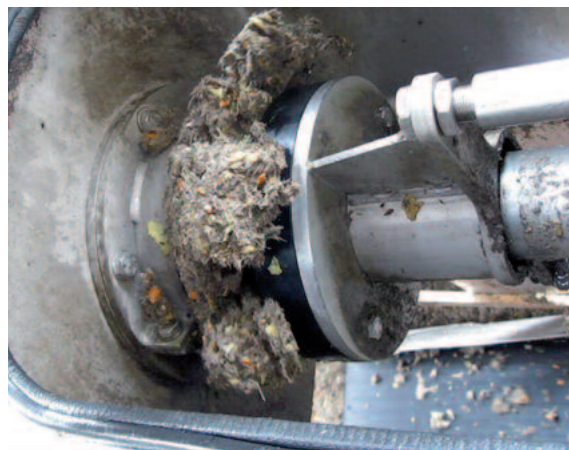
Discharge of the separated pressed material
