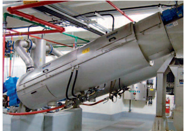
ROTAMAT® Screw Press RoS 3 Specific power consumption < 0.01 kW/kg DR
