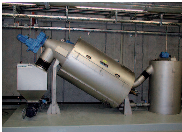
ROTAMAT® Screw Thickener RoS 2 – exceptionally robust thickener
