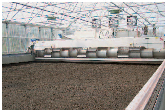
Dewatered sewage sludge becomes dry granulate with the HUBER SRT system
